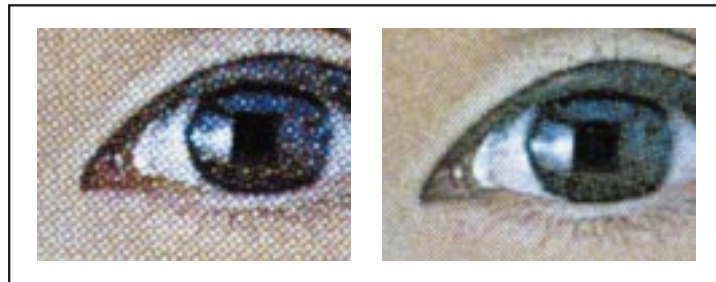
Figure 1 Left: Halftone image (enlarged) produced with conventional technology. The output resolution is 2,438 dpi and the screen ruling is 175 lpi. Right: Halftone image (enlarged) produced with Co-Res SCREENING. Output resolution is the same, but the screen ruling is 300 lpi.
